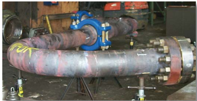
5.1/8" API 15000 psi Flowline under hydro test
