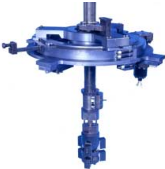
Internal Case Cutting Arrangement
